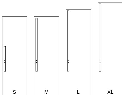
Apart from the classical door closing with door knob or handle with red-/white indicator there is an option available with grab bar, turn lock and integrated LED indicator – especially for classiccell.
