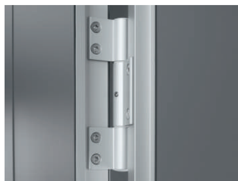
Three-roller edge hinge by KEMMLIT, durable, maintenance free, non-detachable, fastened with six screws
